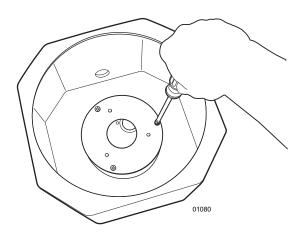
Remove the inside mounting plate by loosening the three Phillips screws.
